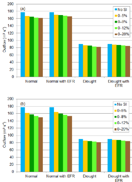
Figure 3. Average annual outflow to Karkkeh dam, before and after supplemental irrigation (SI) withdrawal for four slope classes and four flow scenarios (normal flow, normal with environmental flow requirements (EFRs), drought conditions, and drought with environmental flow); areas that receive both autumn and spring irrigation (a); areas that receive either autumn or spring irrigation or both (b).
