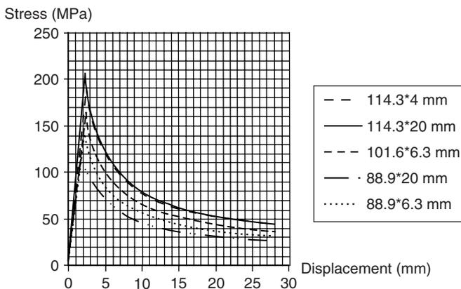
Figure 3. Axial load-axial displacement behavior of the compression members
