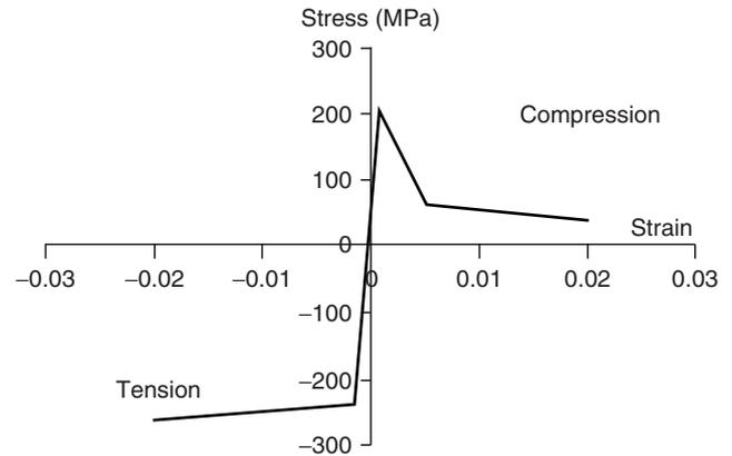
Figure 4. Idealized axial stress-axial strain equation of a sample member in tension and compression
