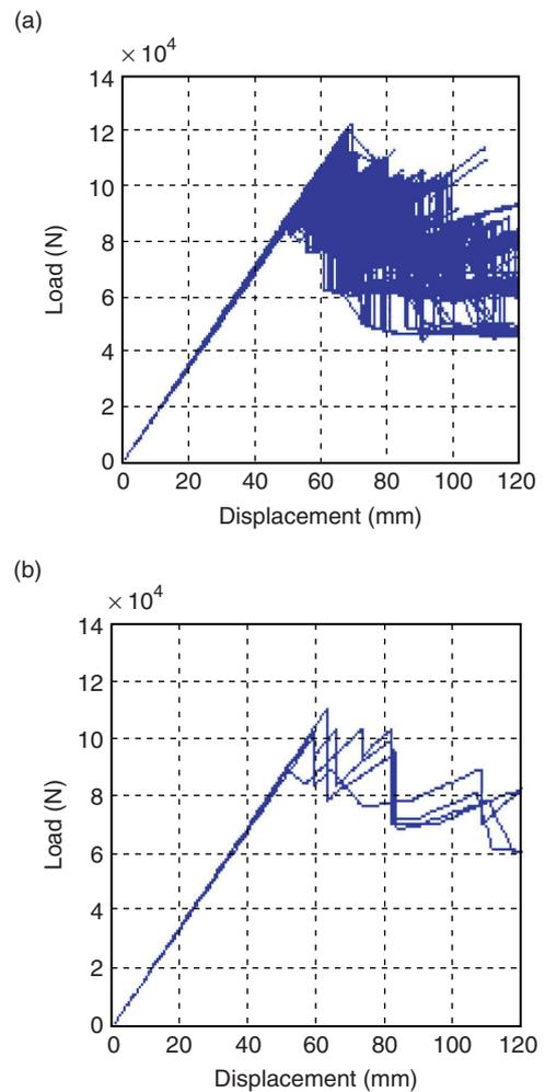
**Figure 8.** Load -displacement diagrams of the double-layer space structure grids: (a) GEd7 all of the samples; and (b) GEd7 some of the samples
