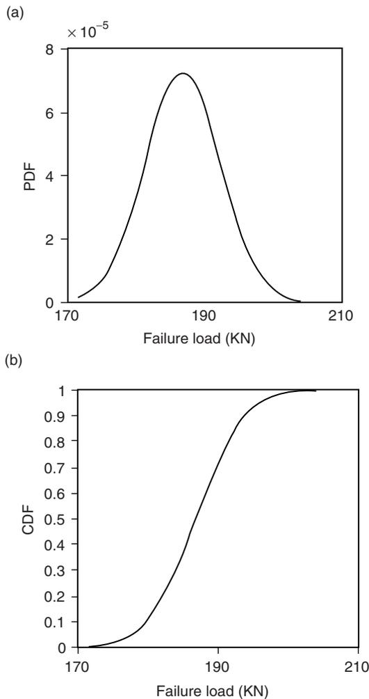
**Figure 13.** Diagrams of the statistical distribution of the collapse load of GS7 double-layer grid: (a) Probability density diagram; (b) Cumulative distribution diagram
