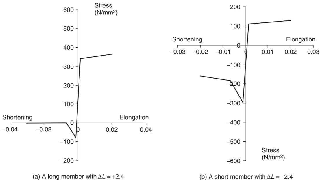
**Figure 7.** Idealized stress-strain relationship of imperfect members under tension and Compression for the type 2 sample with 3 meter length
