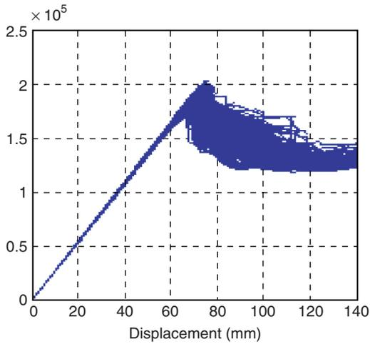
**Figure 10.** Load -displacement diagrams of the double-layer space structure for GS7 grid
