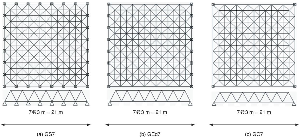
Figure 1. Configuration of the selected double layer grids
