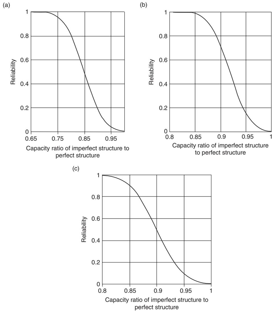
Figure 14. Reliability of the Double layer grids: (a) GEd7; (b) GC7; and (c) GS7
