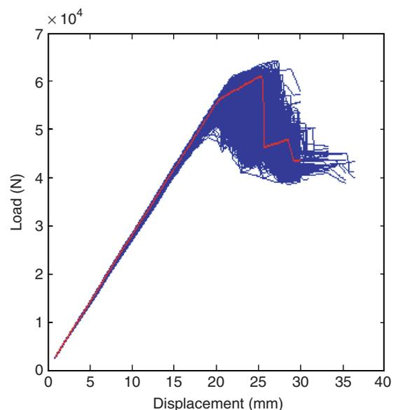
**Figure 9.** Load -displacement diagrams of the double-layer space structure for GC7 grid
