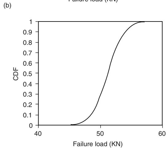
**Figure 12.** Diagrams of the statistical distribution of the collapse load of GC7 double-layer grid: (a) Probability density diagram; (b) Cumulative distribution diagram
