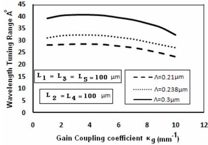
**Figure 4.** Variation of the wavelength tuning rang versus  $\kappa_g$ , ( $\kappa_1 = \kappa_2 = \kappa_3 = \kappa_g$ ).
