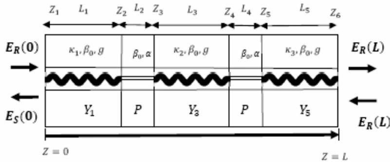
**Figure 2.** Proposed analytical model for GC-2PSC-DFB wavelength-tunable optical.
