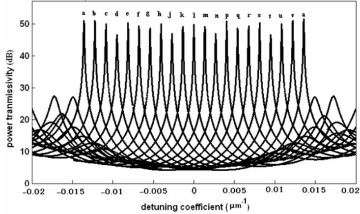
**Figure 5.** Power transmissivity versus detuning coefficient for different values of  $\Omega$  from 0 to  $1.9\pi$  in steps of  $0.1\pi$ . Also,  $\kappa_1 = \kappa_2 = \kappa_3 = \kappa_g = 4\text{mm}^{-1}$ ,  $\lambda_B = 1.55\ \mu\text{m}$ , and  $\Lambda = 0.21\ \mu\text{m}$ . With label l also representing  $\Omega = \pi$ .
