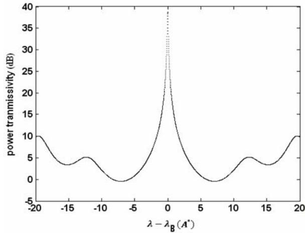
**Figure 3.** Calculated gain profiles of a DFB GC-LD in terms of relative wavelength  $\lambda - \lambda_B$ . Also  $\kappa L = 4.83$ ,  $\lambda_B = 1.55 \mu\text{m}$ ,  $L = 500 \mu\text{m}$  and  $\Lambda = 0.21 \mu\text{m}$ .
