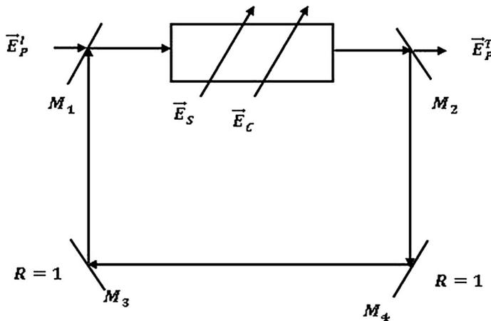
**Fig. 2** Schematic setup of a unidirectional ring cavity with length of  $L$  that consists of the ensemble of  $N$  homogeneously broadened four-level atoms
