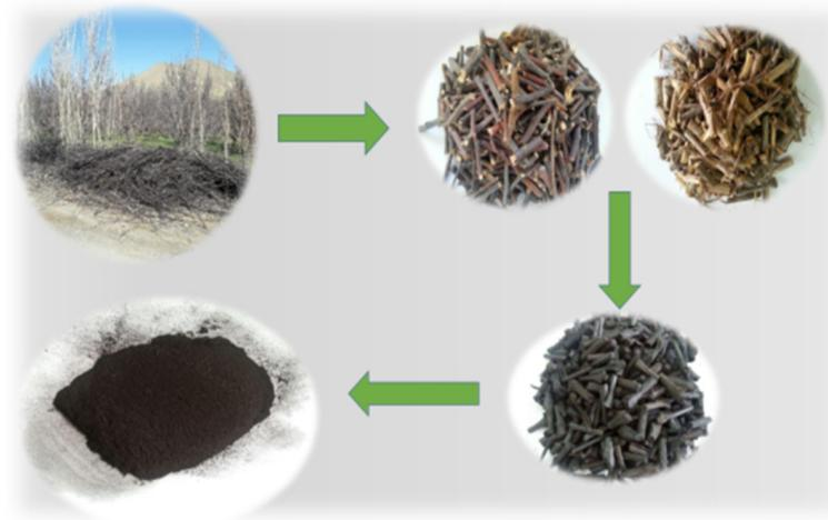
**Figure 1.** Schematic illustration of the preparation of biochar.
