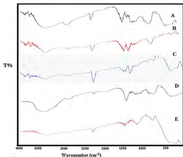
Fig. 3. FT-IR spectra of BC/TiO<sub>2</sub>-Ag (A), BC/PPy (B), BC/PPy/TiO<sub>2</sub>-Ag (C), pure BC (D), and pure TiO<sub>2</sub>-Ag (E).
