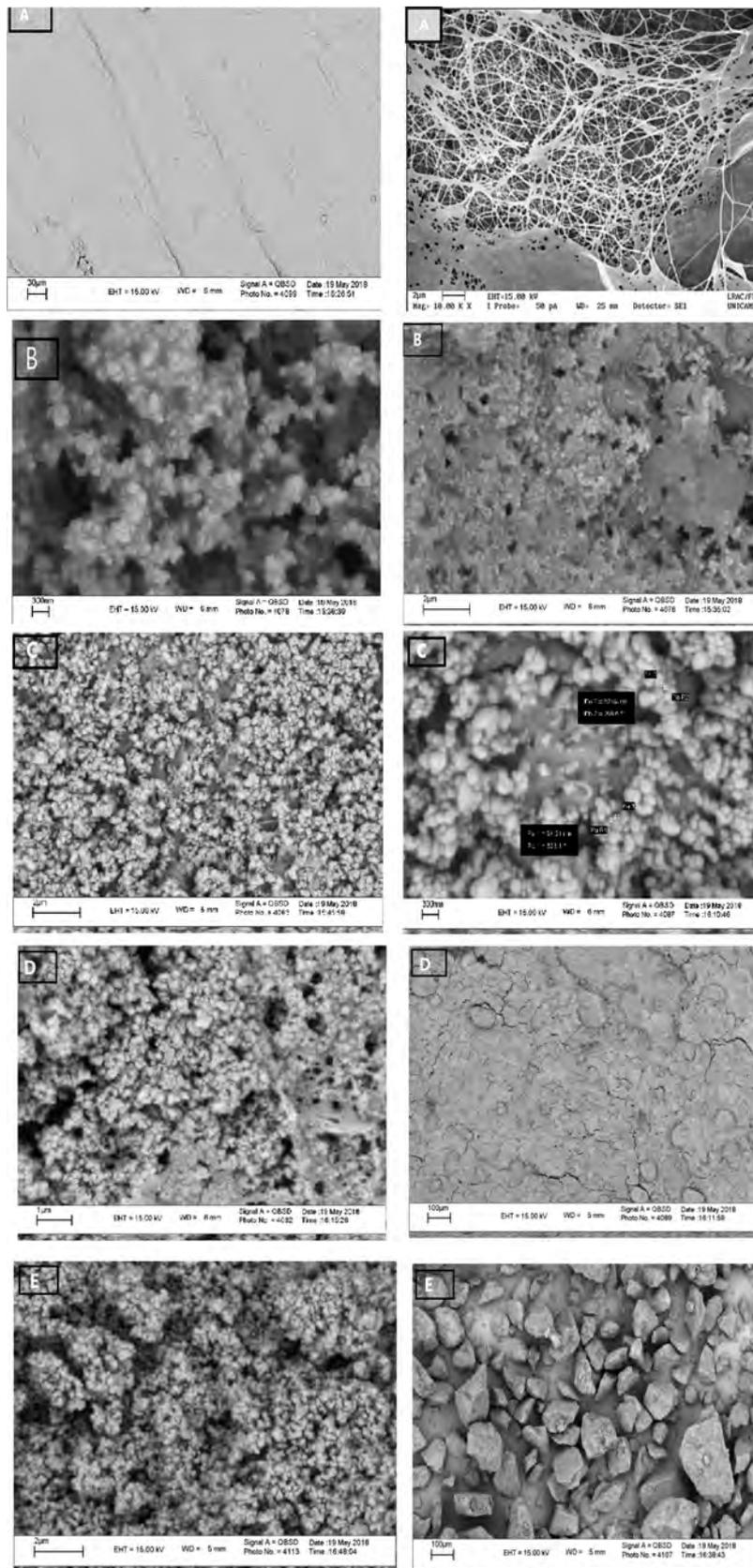
Fig. 2. SEM images of pure BC (A), BC/PPy (B), BC/TiO<sub>2</sub>-Ag (C), BC/PPy-TiO<sub>2</sub>-Ag (D) films and TiO<sub>2</sub>-Ag powder (E).
