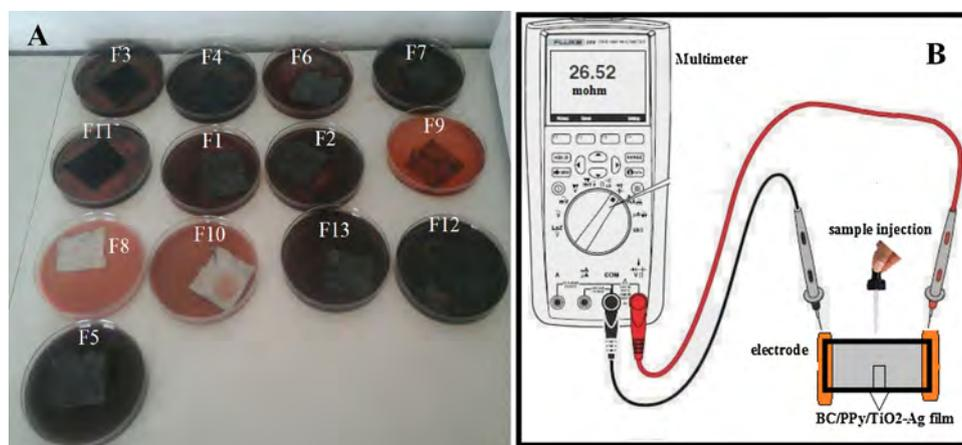
Fig. 1. Different BC, BC/TiO<sub>2</sub>-Ag, BC/PPy and BC/Py/TiO<sub>2</sub>-Ag films (A) and bacteria sample injection system to the sensors (B).
