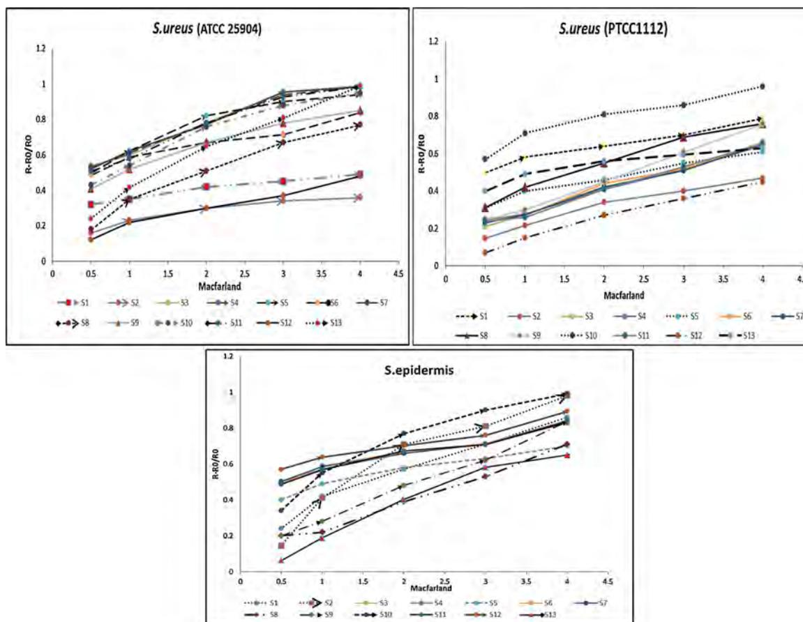
Fig. 4. Response curve of sensors to Gram-positive bacteria.
