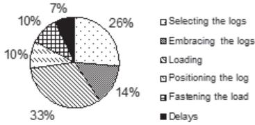
**Fig. 1.** Time consumption distribution of FEL Volvo BM 4500
