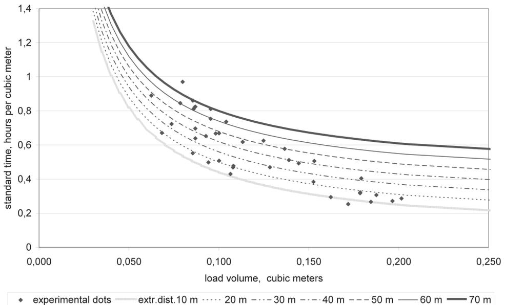
**Fig. 6.** Standard time model, based on load volume
