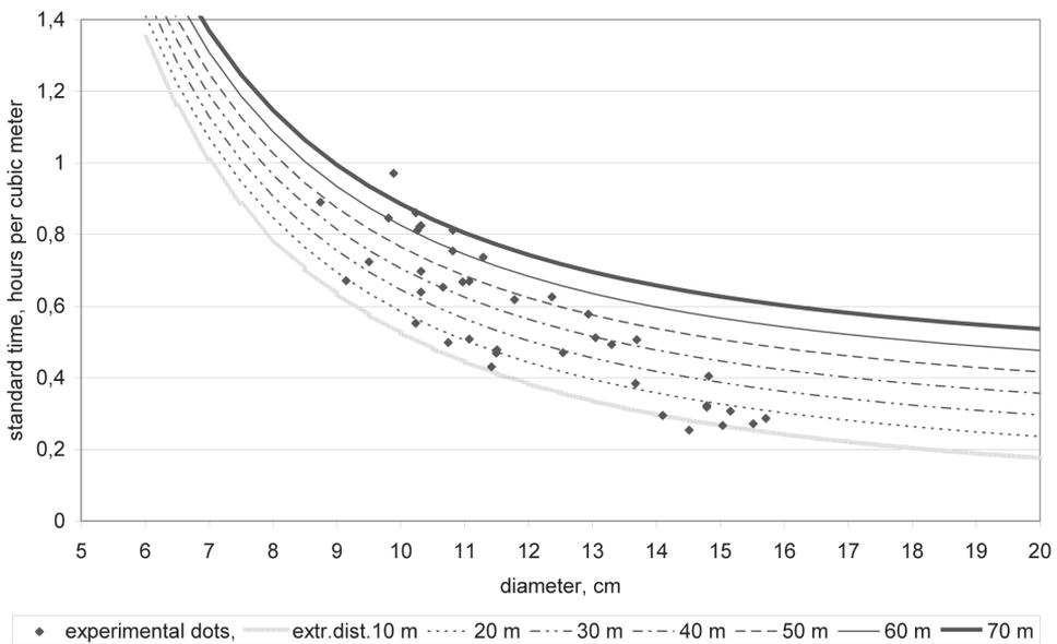
**Fig. 2.** Standard time (time consumption) model, based on mean log diameter
