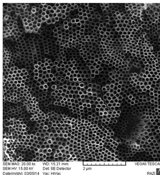
**Figure 2** SEM image of TNTs (conditions for anodisation: water 10%,  $\text{NH}_4\text{F}$  0.35%, 60 V and 4.5 h)
