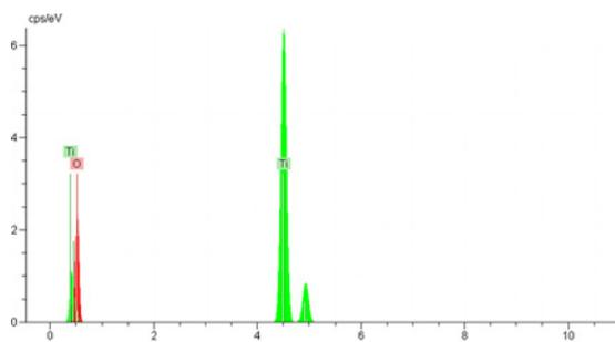
**Figure 3** EDX spectrum of TNTs
