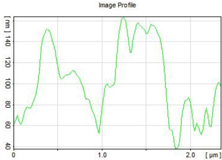
Fig. 6: image profile of Silicon/glass 100 nm layer with an identified length.
