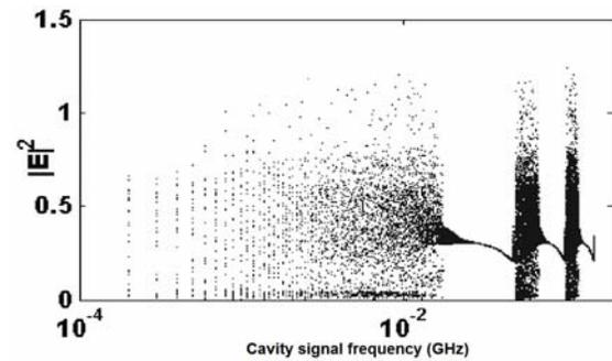
Fig. 3. Bifurcation diagram of the intensity,  $|E|^2$ , Vs. output signal frequency,  $\omega/2\pi$  (GHz), for LEC with  $\tau=121$  and  $T=550$ .
