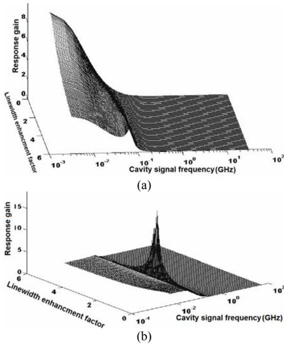
Fig. 5. Response gain of carrier number versus  $\alpha$  and  $\omega/2\pi$  (GHz) for a) LEC and b) SEC.
