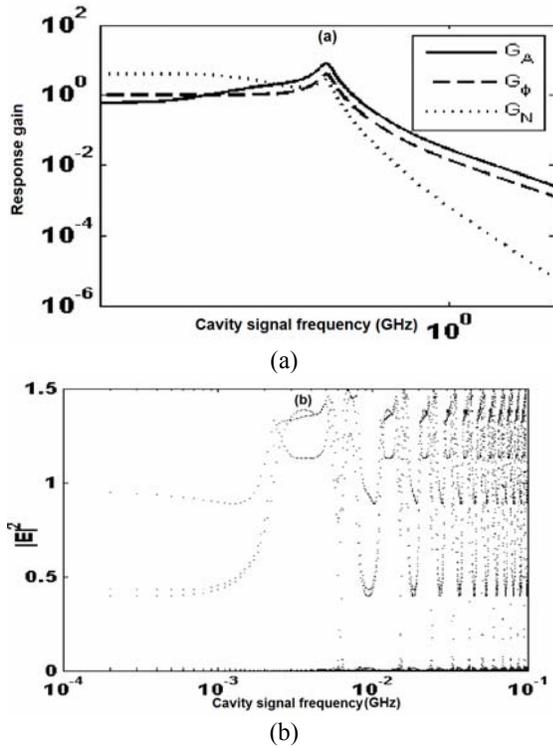
Fig. 1. a) Response gain of LEC, (Thick, thin, and dotted lines are correspond with responses in field amplitude, optical phase and carrier number, respectively), and b) Bifurcation diagram of the intensity,  $|E|^2$  versus signal frequency output,  $\omega/2\pi$  (GHz), for LEC with  $\tau=700$  and  $T=300$ .
