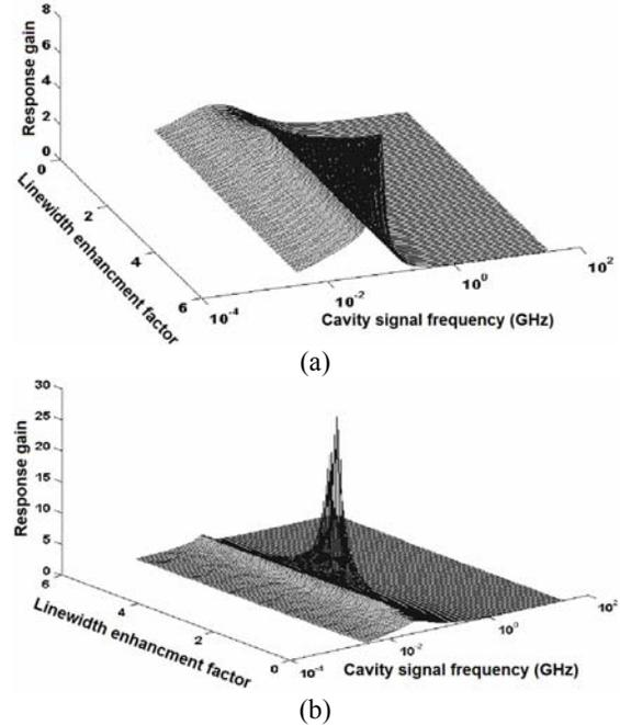
Fig. 4. Amplitude response gain against  $\alpha$  and  $\omega/2\pi$  (GHz) for a) LEC and b) SEC.
