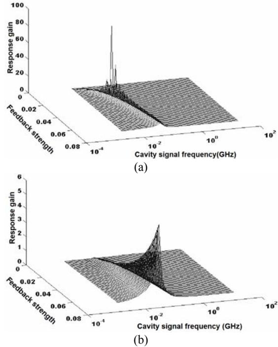
Fig. 6. Response gain of amplitude versus  $k$  and  $\omega/2\pi$  (GHz) for (a) LEC and (b) SEC.
