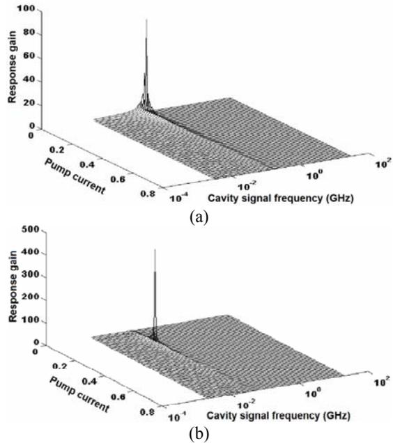
Fig. 7. Response gain of amplitude versus  $P$  and  $\omega/2\pi$  (GHz) for (a) LEC and (b) SEC.
