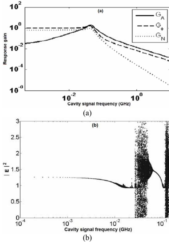
Fig. 2. a) Response gain of SEC, (Thick, thin, and dotted lines are corresponding with response in field amplitude, optical phase and carrier number, respectively), and b) Bifurcation diagram of the intensity,  $|E|^2$  versus the output signal frequency,  $\omega/2\pi$  (GHz), for SEC with  $\tau=70$ ,  $T=1710$ .
