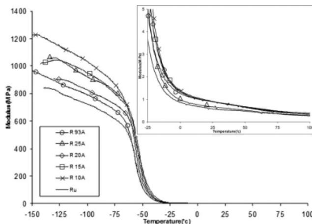
**Figure 3** Storage modulus of nano-composites and the base compound.
