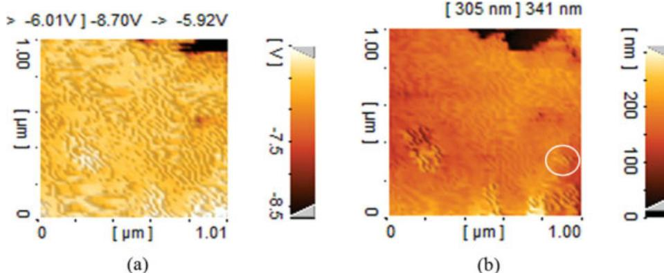
**Figure 5** AFM micrographs from the surface of R10A nano-composite (a) phase image (b) height image. [Color figure can be viewed in the online issue, which is available at [www.interscience.wiley.com](http://www.interscience.wiley.com).]
