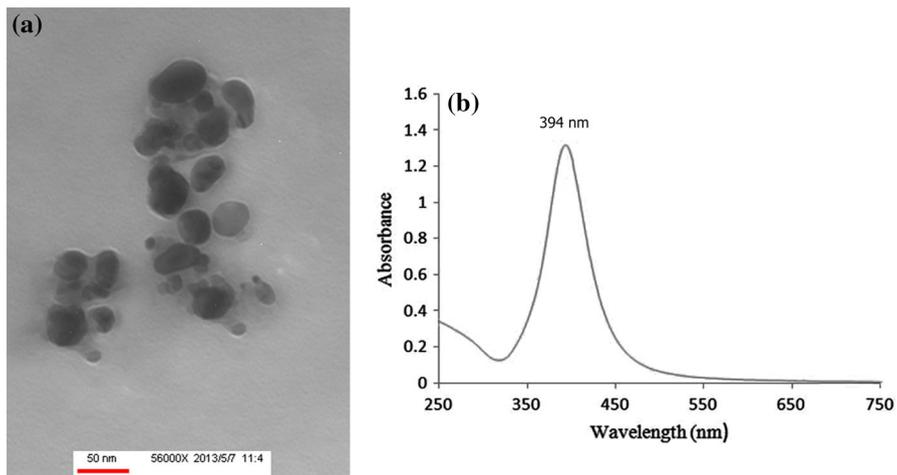
**Fig. 1** **a** Transmission-electron micrograph of silver nanoparticles employed in the present study. **b** Formation and the stability of silver nanoparticles in aqueous colloidal solution are confirmed using UV-Vis absorption spectrum of AgNPs
