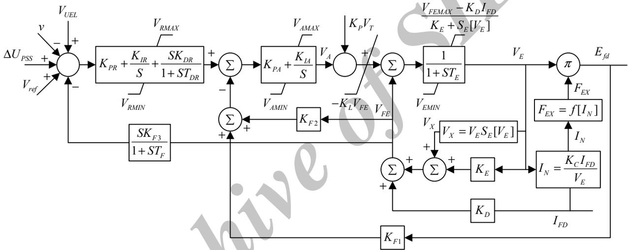
Fig. 5. IEEE type AC7B brushless excitation system model [5].
