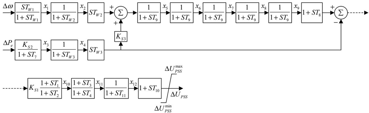
Fig. 8. Assign new state variables to dual-input PSS2B stabilizer.
