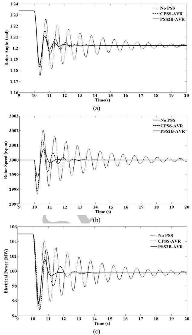
Fig. 14. System heavy responses for mechanical power disturbance, (a) rotor angle, (b) rotor speed, and (c) machine active power.
