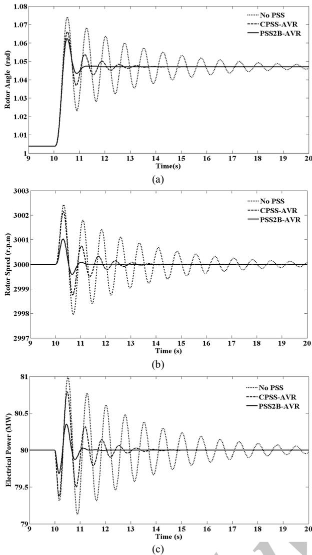
Fig. 13. System light responses for reference voltage disturbance, (a) rotor angle, (b) rotor speed, and (c) machine active power.
