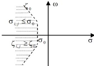
Fig. 9. Desired sector for repositioned eigenvalues.
