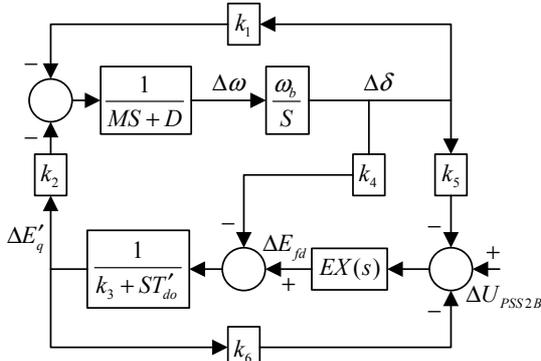
Fig. 7. Phillips-Heffron model of the steam unit equipped with PSS2B.
