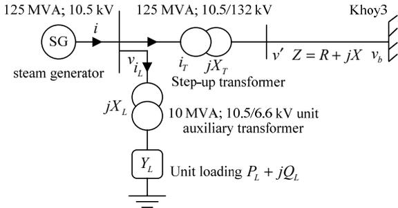
Fig. 3. Single line diagram of the steam unit.
