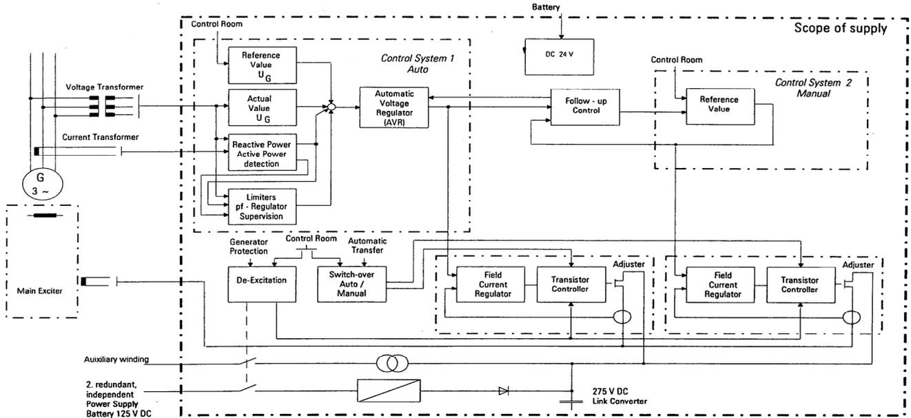
Fig. 4. Single line diagram of the RG3 excitation system for the steam unit [8].
